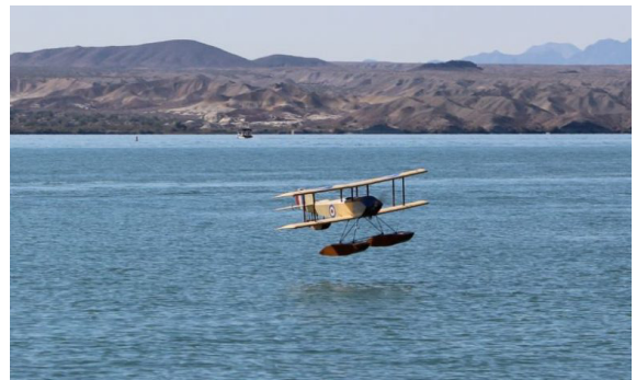
(Above) A Sopwith Schneider Baby built by Marjoe Bunney comes in for a landing. 108-inch span, 46lbs. and Quadra Q-100 for power.
