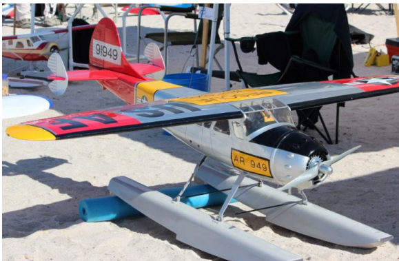
(Above) Aeroworks Cessna 195 flown by Larry Ayotte of Mesa Arizona. 90 inch wingspan, 21lbs. and powered by a DLE 35.
