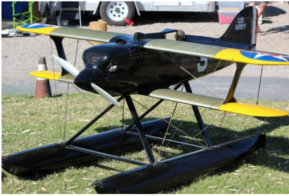
(Above) One of the Schneider cup racers. This one is a Curtiss R3C-2. The full-scale was flown by Jimmy Doolittle in the 1925 Schneider cup race. This model was built by the team of Larry Tate, Jerry Lieche, John Hanks and Bob Martin in 1988. 88-inch wingspan, 39 lbs. and powered by a Sachs 4.2ci engine.
