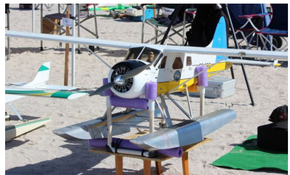
(Above) Carlos Rangel of Tucson brought his Top Model Beaver. Electric power using an E-Flite 150 and 10 cell Li Po battery pack. 1/5 Scale model has a 90" wingspan.
